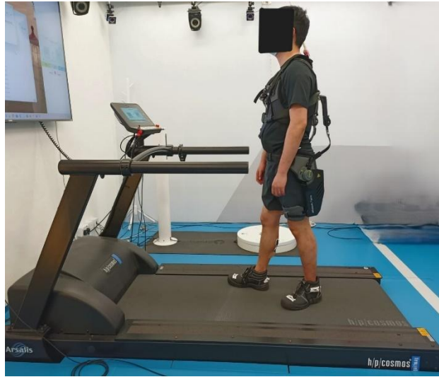
Figure 2. Participant walking on the treadmill integrated with force plates.
