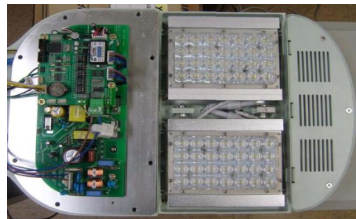
Fig.7. Smart LED Light Panel using ZigBee Protocol
